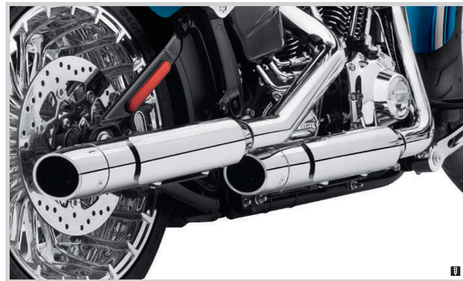
E. SCREAMIN' EAGLE STREET CANNON SLIP-ON MUFFLERS – SOFTAIL SHORTY DUAL, CHROME (SHOWN WITH BILLET CHROME END CAPS)
